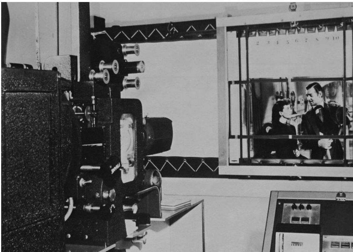
The conversion of the original 35mm print of GWTW to its attenuated 70mm form.
